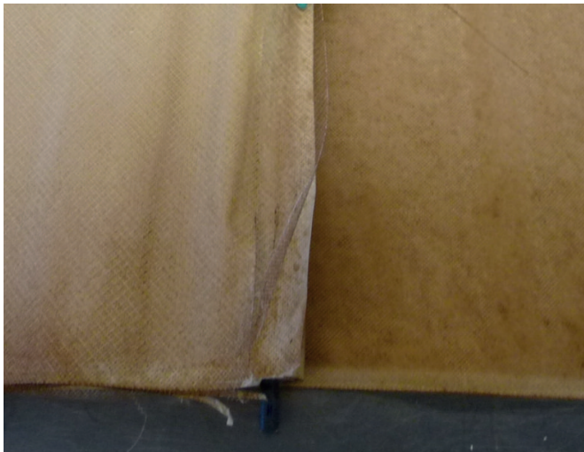
Figure 6: Comparison: Membrane surface of the ASD element on the left, standard spacer on the right.
