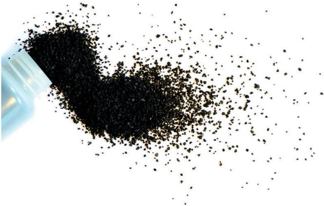
Figure 2: Granulated activated carbon (GAC) (Source: IWW)
