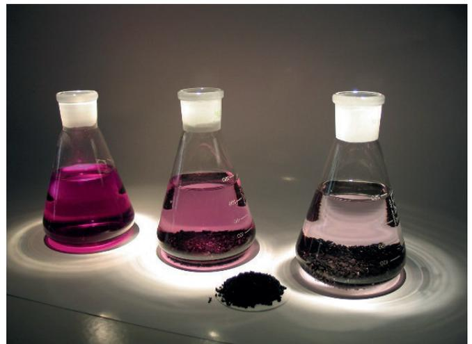
Figure 1: Discolouration with activated carbon (Source: IWW)
