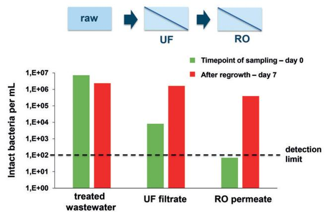
Figure 3: Concentrations of inactive bacteria in the effluent (raw water), resp. after undergoing the ultrafiltration (UF) and the reverse osmosis (RO) processes on the day of the water sampling (Day 0, green bar), resp. after bacterial growth (Day 7, red bar). The detection limit of flow cytometry is at about 100 bacteria per mL.
