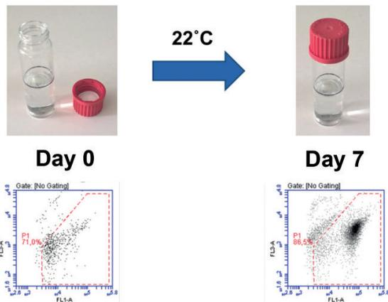
Figure 2: Exemplary presentation of determination of growth potential. The growth is measured by the difference in bacteria numbers on day 0 and day 7. The multiplying factor shows the growth potential that can occur under defined temperatures in stagnant water in the worst case.
