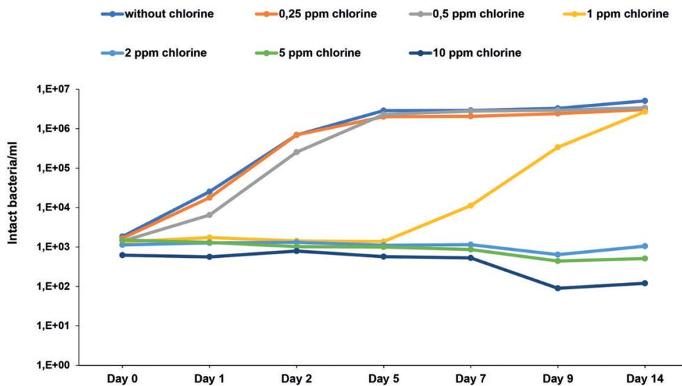
Figure 4: Determination of the sustainability of different chloride concentrations (hypochlorite) on the bacterial growth in UF permeate via flow cytometry.
